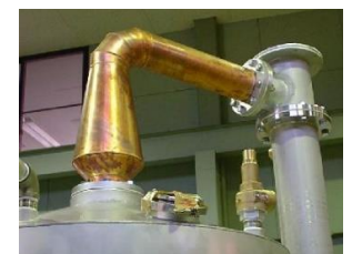
Copper (optional) inside the gooseneck and condenser
