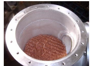
Copper (optional) inside the gooseneck and condenser
